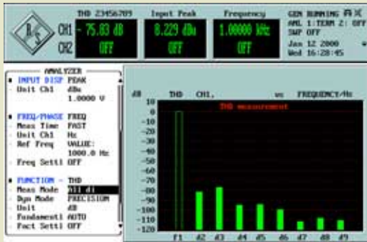
Fig. 2: THD measurements can include single harmonics, all harmonics or any combination of harmonics.
